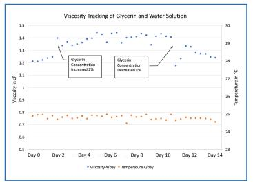
Illustration 2, demonstrates that the ViscoPro 2100 provides stable results over long periods. The viscometer is sensitive to very small changes in viscosity. The piston motion provides adequate mixing and sample exchange in non-agitated tank.
